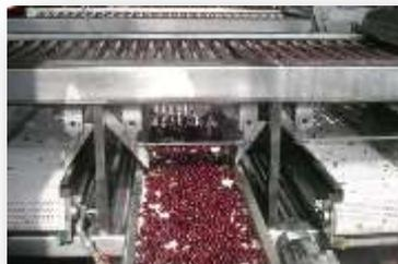
surplus levels of product on the calibration rolls are removed, thus leaving **always only one level (or row) of the product on calibration rolls** - the first condition for a perfect calibration
